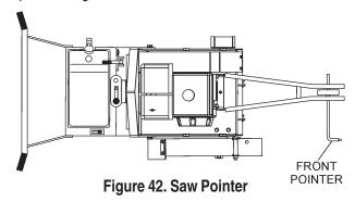
To reorient a pointer position, loosen the screw that secures the pointer bar to the shaft, adjust as necessary, and retighten the screw.
